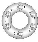
13. Tighten the nuts firmly in a crisscross sequence, as shown, by turning the wheel wrench clockwise.
