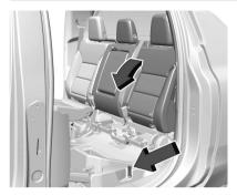
Pull the release strap located below the seat cushion to unlock the seatback. Fold the seatback forward and down.
