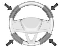
Super Cruise steering can be overridden with manual steering at any time. To begin steering manually, hold the steering wheel firmly with both hands.
