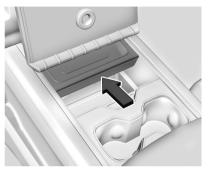
To access additional floor console storage, the USB port, and the auxiliary power outlet, slide the wireless charger forward until it stops, then release to lock it in place.
