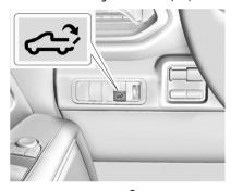
• If equipped, press on the instrument panel to the left of the steering wheel.
