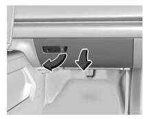
To open the glove box, pull the handle to the left. Use the mechanical key to lock or unlock. See  $Keys \Rightarrow 6$ .
