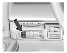
The Electric Parking Brake (EPB) can always be applied, even if the vehicle is off. In case of insufficient electrical power, the EPB cannot be applied or released. To prevent draining the battery, avoid unnecessary repeated cycles of the EPB.
