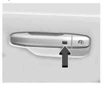
The remote key must be within 1 m (3 ft) of the eTrunk or door being opened or locked. Press the button on the door handle to open. See "Keyless Access Operation" in Remote Key Operation ▷ 7.
