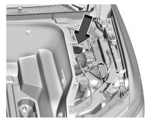
4. After the system has completely cooled, check that the coolant level in the reservoir.
