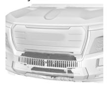
The vehicle may have a shutter system that automatically closes the frontal cooling openings. This system promotes airflow around the vehicle, reducing drag and providing energy savings. Ensure the shutter
