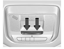
The front reading lights are in the overhead console
