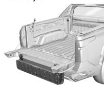
To close the inner tailgate with the primary tailgate closed, firmly push or pull it upward until it latches. Pull or push it back to be sure it is latched securely.
