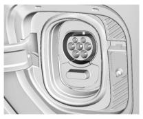
When the charge cord is plugged in, a color indicates the charging status.
