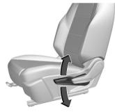
If equipped, move the lever up or down to manually raise or lower the seat.
