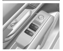
The power windows work when the ignition is on, in accessory mode, or when Retained Accessory Power (RAP) is active. See *Retained Accessory Power (RAP)* ⇔ 162.
