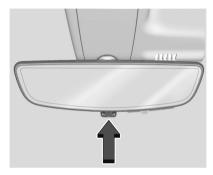
Pull the tab to turn on the display. Push the tab to turn it off. When off the mirror has automatic dimming. Adjust the mirror for a clear view of the area behind the vehicle while the display is off.
