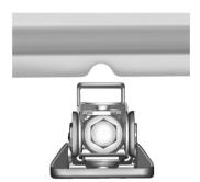
9. Position the jack lift head at the jack location nearest the flat tire. The location is indicated by a notch in the vertical bottom edge of the body side sheet metal.
