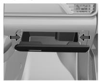
2. Squeeze both sides of the glove box bin inward to lower beyond the stops.
