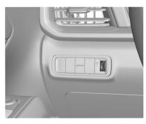
This feature adjusts the brightness of all illuminated controls. The instrument panel illumination control is next to the exterior lamp control.
