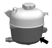
Check to see if coolant is visible in the coolant surge tank. If the coolant inside the coolant surge tank is boiling, do not do anything else until it cools down. If coolant is visible but the coolant level mark is not visible, add a 50/50 mixture of clean, drinkable water and DEX-COOL coolant at the coolant surge tank to the top rib on the middle of the tank, but be sure the cooling system is cool before this is done. See Engine Overheating \$\triangle\$ 228.
