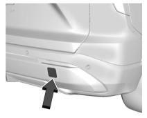
If equipped, carefully open the cover by using the small notch that conceals the rear tow eye socket.
