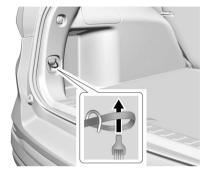
Route the loop end of the strap through one of the cargo tie-downs in the rear of the vehicle.
