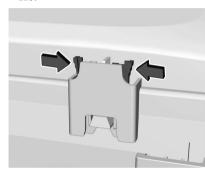
To remove the fuse block cover, squeeze the clips on the cover and lift it straight up.
